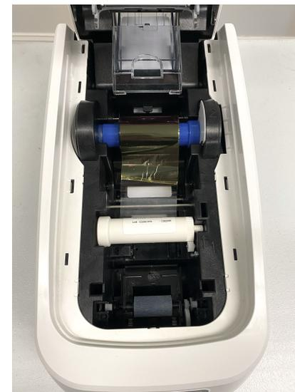
Insert new film. The blue spool goes in the back, left side first. Closer printer. Hit retry on the screen.
