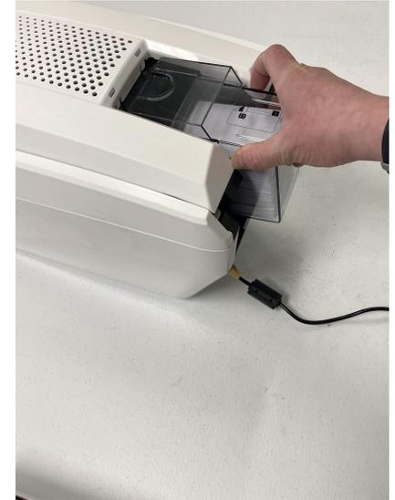
Replace hopper firmly in the back of the printer. Hit retry on the screen.
