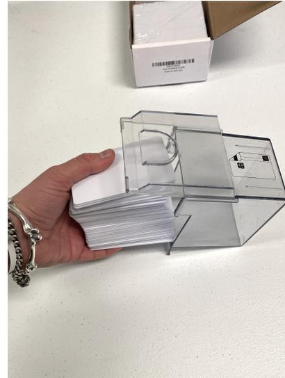
Unwrap one pack of cards from the box and place them in the hopper. Make sure the hopper is facing up right. The hopper can only hold 100 cards at a time.
