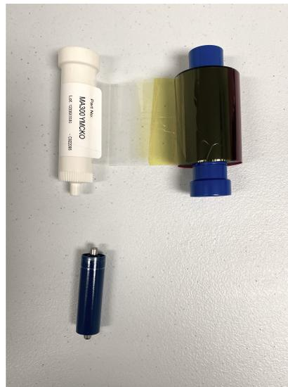
Remove protective film from cleaner roll. Pull film spools apart from one another. Insert metal spindle through center of new cleaner roll.
