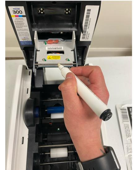
Use the pen to gently remove debris from the printer head. Replace all cards and film in printer. Press retry on front screen if necessary.
