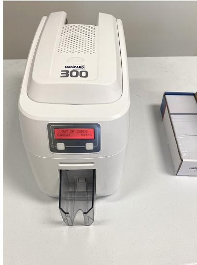
When the printer screen says out of cards it is time to replace the cards.
