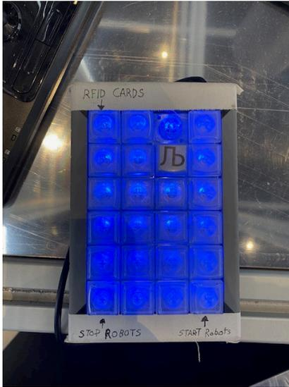
Press button labeled RFID cards to switch into reactivation mode.
