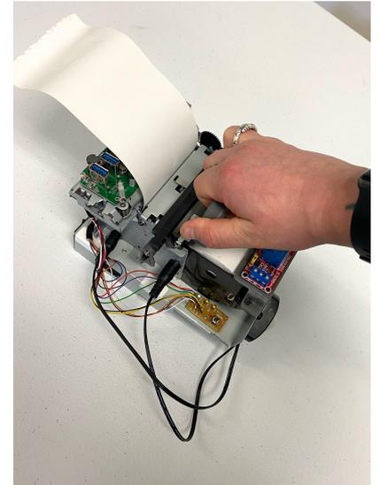
Replace bracket over top of paper by pushing it in from the top and then pulling back (reverse motion of taking it out). Make sure that the gears on the side are aligned.
