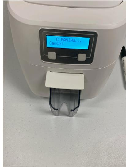
The printer will pull the card in and run a cleaning cycle.
