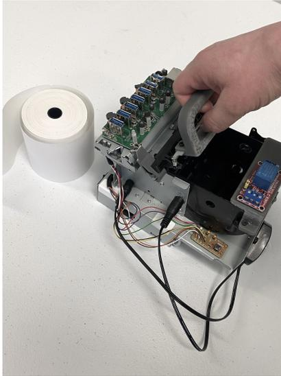
Remove top bracket by pulling handle up at a 45 degree angle...
