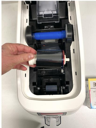
Open printer by pressing top button and remove old film, both the white and blue spools.
