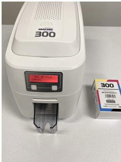
When the printer screen reads "out of film" it is time to replace the film.
