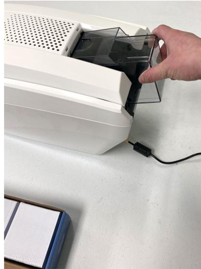
Remove the card hopper from the back of the printer.
