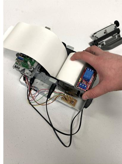
Be sure to remove old printer paper before placing paper into opening. May be a tight fit at first, unroll some paper if needed.
