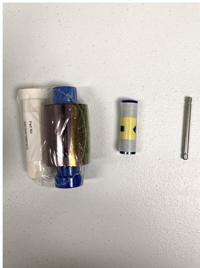
Discard old film and spool, but keep metal spindle. Take replacement film and spool out of the box.
