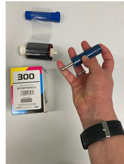
Push metal spindle out from center of cleaner roll.
