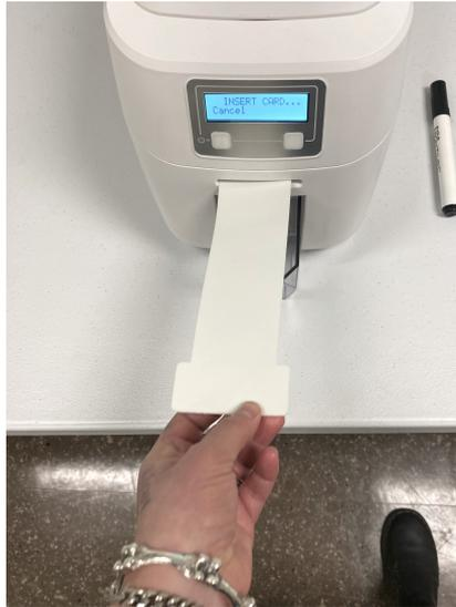
When prompted insert the cleaning card into the printer with the T side facing out.
